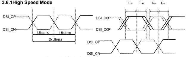
Figure 1: DSI clock timing Characteristics
