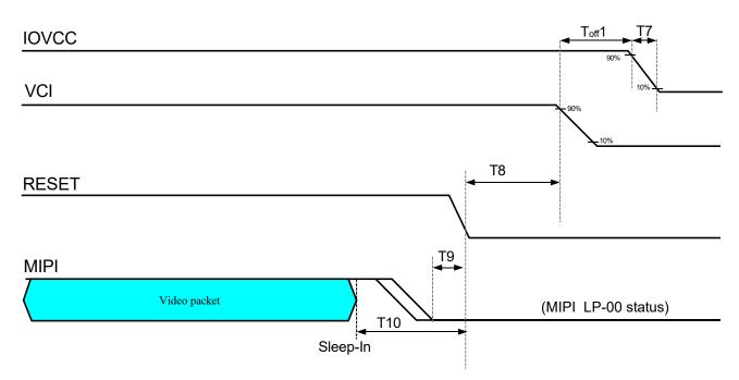
Figure 4 Power off sequence at PCCS[1:0]=[1,0] mode
