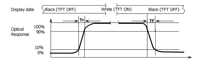
Figure 4-4 Response Time Testing
