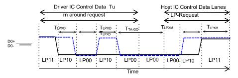
Figure 2: BTA from Display Module Timing to HOST
