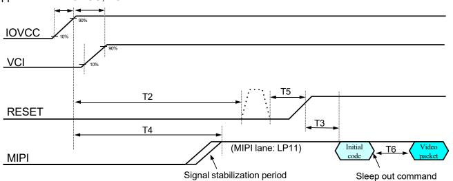
Figure 3 Power on sequence at PCCS[1:0]=[1,0] mode
