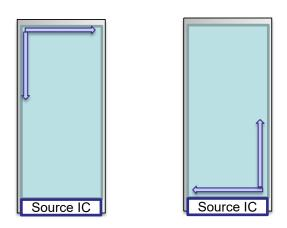
Figure 3-1 The U/D direction setting
