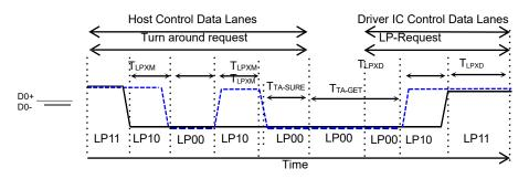
Figure 3: BTA from HOST to Display Module Timing
